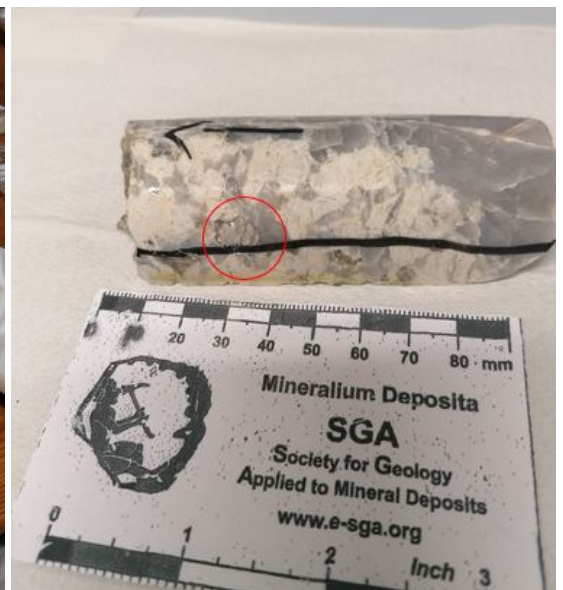
Photos: Spectral measurements were conducted in surface (left) and drill-core samples (right), from Norway and Ireland, respectively. The figure on the left also shows the software for collecting the spectra, while the sample photograph on the right shows a red circle indicating the spot analyzed. (Photos: UPORTO)
